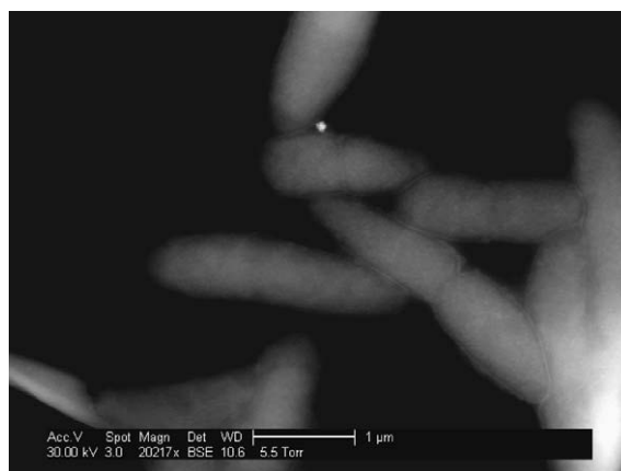
Fig. 11. Annular dark-field wet STEM image at 30kV of organic objects submerged in a liquid phase: Pseudomonas syringae pv. Syringae bacteria, strain PPI203: double membrane structure and cellular division are observed.
