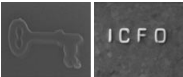
Figure 5 and 6: A “golden nano-scale key” deposited with the Nova™ 600 NanoLab using the direct bit-map writing facility (left) and the continuous writing of the ICFO name (Institute of Photonic sciences, Barcelona, Spain) using a Quanta™ 200 with Elphy Plus from Raith GmbH (right). The start of the (repeated) writing pattern (Fig 6) results in a slightly lower local deposition, which is probably due to the start-up of the surface diffusion process.
