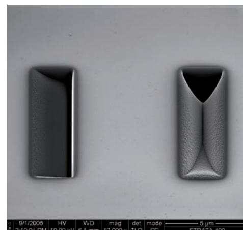
Fig. 15: when the patterning is done in a single pass (e-beam lithography style) pronounced artifacts are present for both sweep directions.
