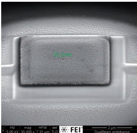
Fig. 3: intermediate step of a crossbar architecture intended for self-assembly of alkanethiol based functional molecules. Bright 5 μm square with leads to either side: W deposition; concealed square: Au deposition; covering layer: insulating SiO x . 50 nm FIB-milled hole to the Au in the center.
