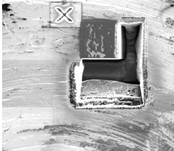
Fig. 2: Example of automated sequential FIB slicing and EDS map collection a standard Al stub for electron microscopy. The volume analyzed is 20 \times 16.6 \times 20.3 \mu\text{m}^3 .
