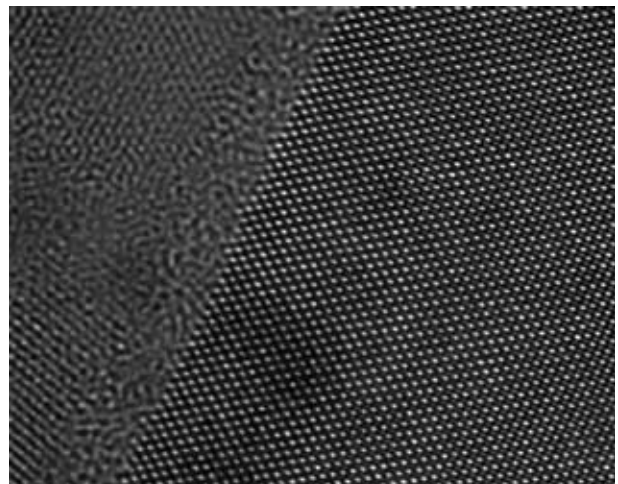
Image of a gate oxide in a semiconductor device – taken with a Titan with image Cs corrector on at 80 kV. This is particularly significant since this voltage is below the damage threshold in carbon. The information limit at this voltage was still below 1 nm.
