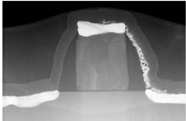
Sample thinned to a transmission sample for in-chamber STEM and EDS analysis, showing titanium-rich material shorting out the gate.
