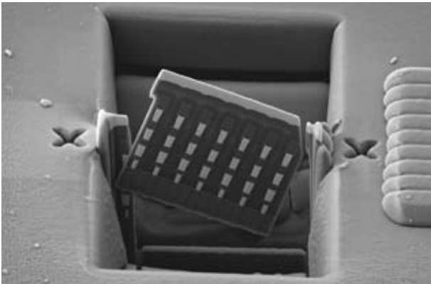
A thinned section prepared by FIB automation for TEM is ready for ex-situ lift-out.
