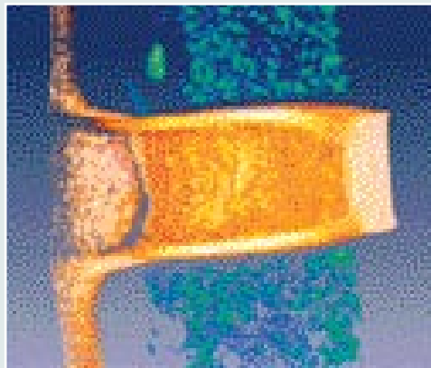
3D image of Copper Contact with surrounding porous SiLKTM resin. Sample Courtesy: The Dow Chemical Company and IMEC, Leuven, Belgium
