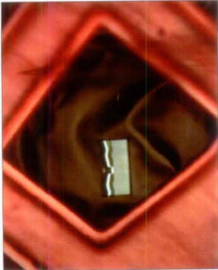
Fig. 6. Image showing a FIB-prepared foil in a copper TEM sample grid.
