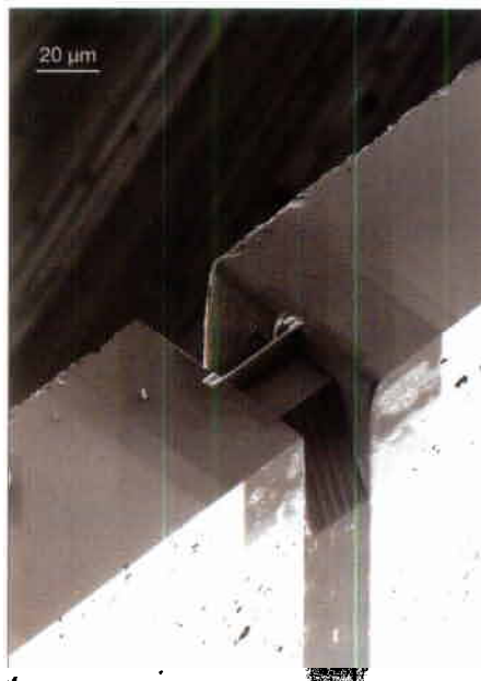
Fig. 4. The sample in this image was mechanically pre-thinned before being placed into a FIB system where the thin foil in the center was machined.
