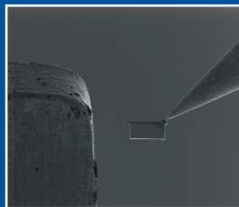
TEM sample moved to waiting TEM grid.
