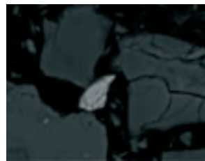
A backscattered image of a FIB section through a rock sample.
