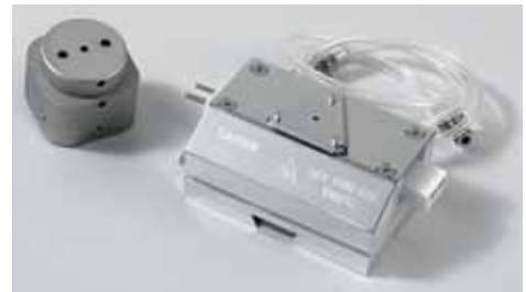
Optional 1000°C Heating Stage for heating bulk samples.
