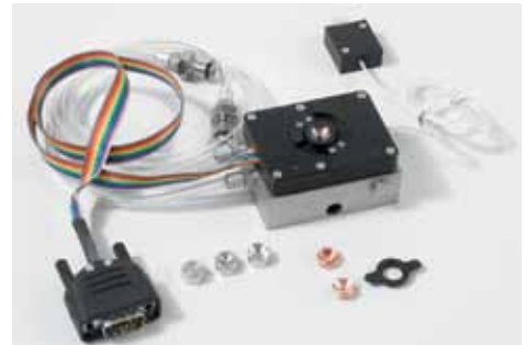
Optional WetSTEM™ cooling stage for bulk samples (like the Peltier cooling stage) and thin or electron beam transparent samples.
