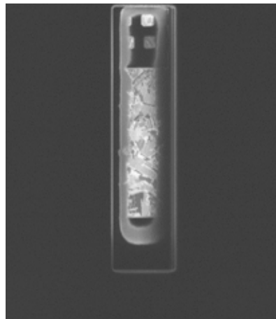
Fig. 2a: A second opening exposes the copper bus line between the jumper and the ground source. The jumper, further down the bus line, is not in the field of view.
